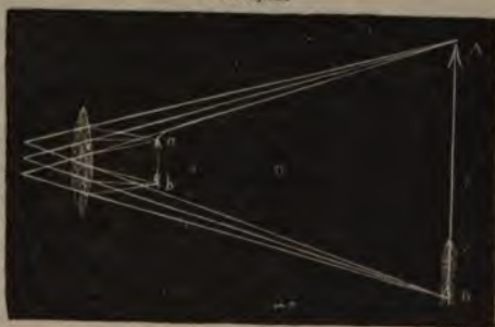
Diagram illustrating the action of the Simple Microscope ; a b object; A B its magnified image.
